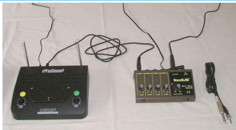
Figure 4. Photo showing connection between units.
