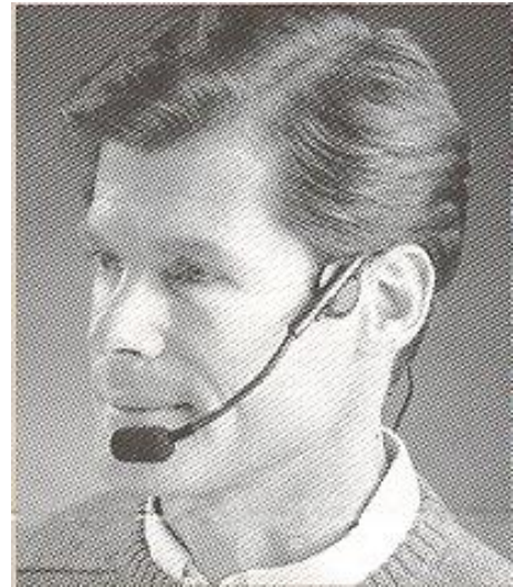
Figure 9. Recommended mounting position for Head Mounted Mic. This is what it looks like with the windscreen removed.
